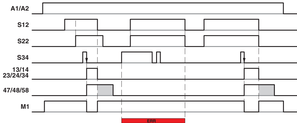
Figure 7 Time diagram for off delay, manual start
